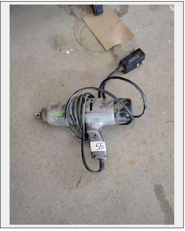
**Description** This is a used Ingersoll Rand Impactool, Model 8055. This 3/4" impact tool runs on 120 volts AC/DC. It runs at 1750 RPM.
