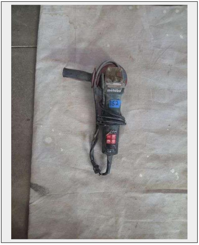
**Description** Metabo WE 15-150 Quick Angle Grinder with 13.5 amp motor and 6" diameter wheel. Automatic safety system and quick wheel change.
