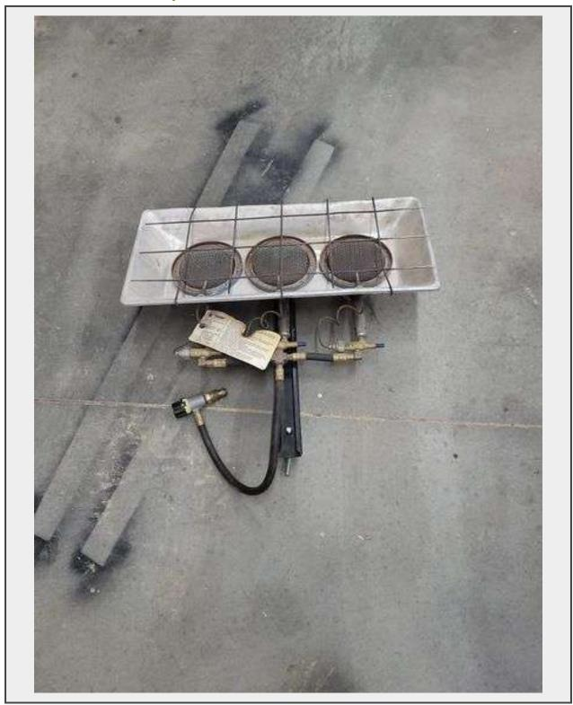
**Description**Mr. Heater Corp. propane heater with three burners and fittings for propane tanks.
