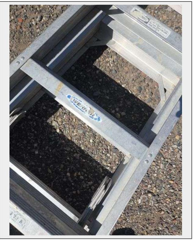
**Description** Werner T408 Aluminum Ladder. It's a Duty Master Extra Heavy Duty industrial ladder, with a 300lb weight capacity.
